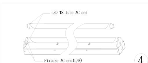
4. Put the LED T8 tube into the fixture. Make sure the AC end of the LED tube matches the AC end of the fixture. When the LED tube is installed in, turn the tube left or right by 90° to make sure the tube is secured in the fixture. (Note: Find out the AC end of the LED tube before install it into the fixture.)
