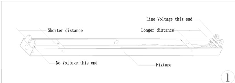
1. Install the socket into the fixture.
