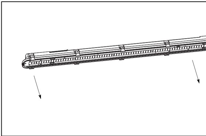
6. Locate safety cable when opening to install fixture body and snap connect tether to gear tray before making electrical connection as shown in figure.
