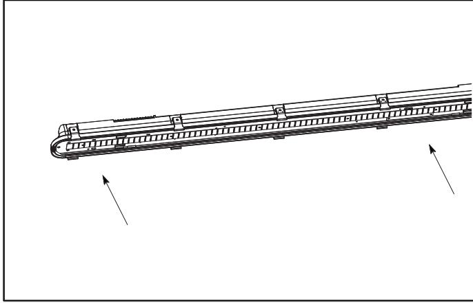
9. Secure lens to housing with lens latches.
