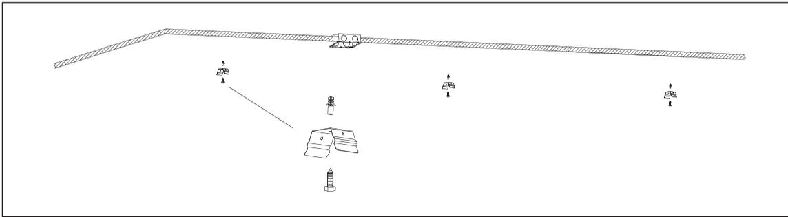
2. Secure mounting clips to housing recesses by firmly pressing them into place until both sides of the clip are secured.
