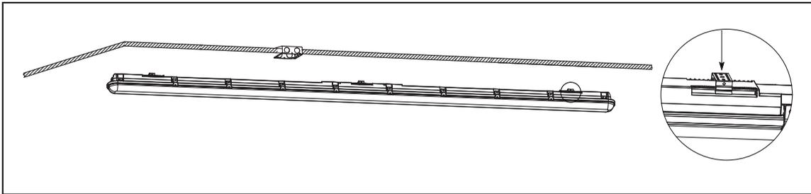
3. Release latches by pulling top of latch away from housing.
