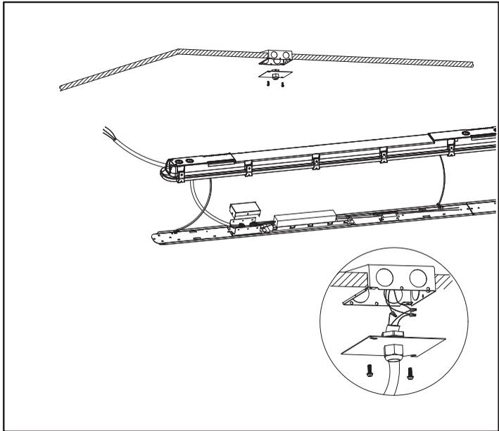
9. Reattach LED tray to fixture by reversing step 5.
