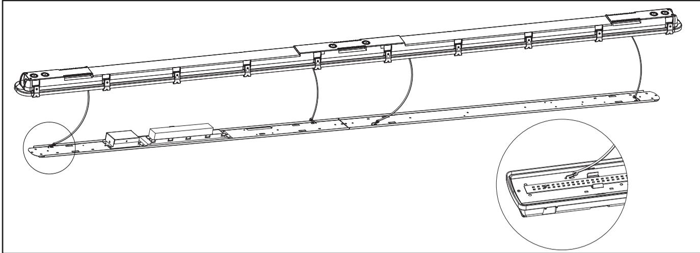
6. Connect power supply to the driver through the outlet box as shown in the figure (the flexible cord is customer supplied), make sure to snap the cover to the outlet box after wiring is completed.
