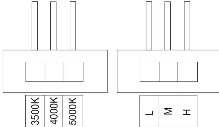
The end users may adjust the color temperature and lumen output respectively by the two DIP switch. Each DIP switch is accommodated with 3 options (left, middle and right), corresponding to 3 color temperatures and 3 powers respectively, which can perform the desired color temperature and lumen output combination.
