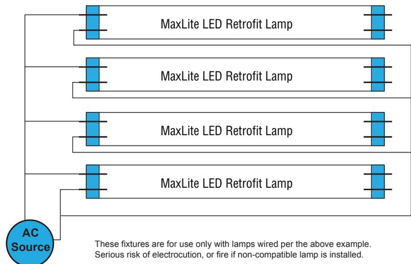
These fixtures are for use only with lamps wired per the above example. Serious risk of electrocution, or fire if non-compatible lamp is installed.
