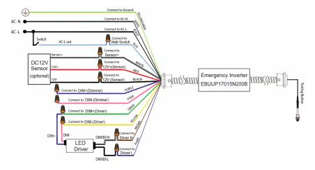
3. For luminaire with non-dimming LED driver (\* LED DRIVER INPUT POWER NOT GREATER THAN 15W)
