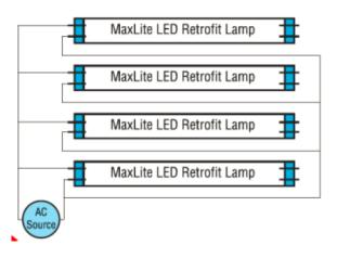
These fixtures are for use only with lamps wired per the above example. Serious risk of electrocution, or fire if non-compatible lamp is installed.
