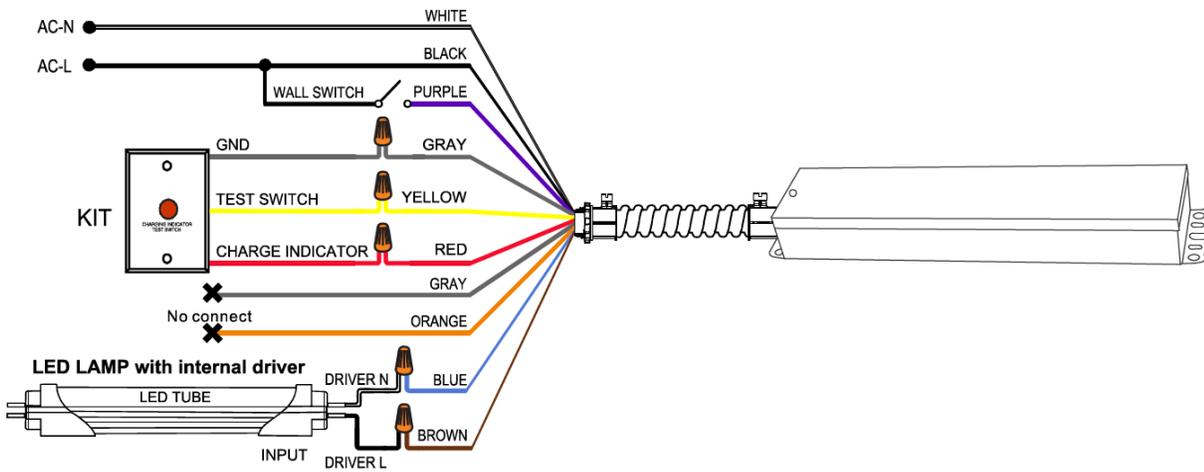
2. When LED driver power is more than emergency power and 0-10V wall switch is installed.
