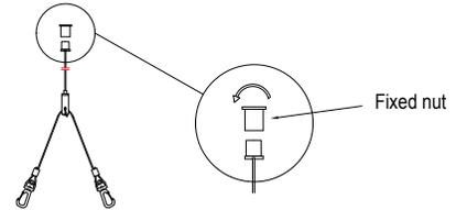
Step 3 : Fasten the retaining nuts to the retaining frame with screws.
