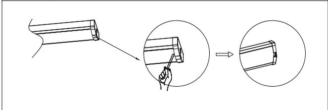
Step 3: Remove the Lens and the protective film from lens.
