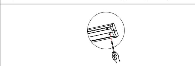
Step 6: Tighten the screws to complete back shell installation.
