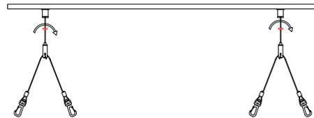
Step 5 : Hang the rope hook into the lamp body.
