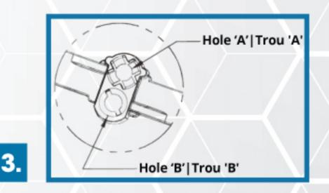
**STEP 1:** Attach the mounting bracket to a 3½" or 4" round or octagonal box with the screws provided. The "A" side of the bar is for a flat ceiling and the "B" side is for an uneven or textured ceiling.
