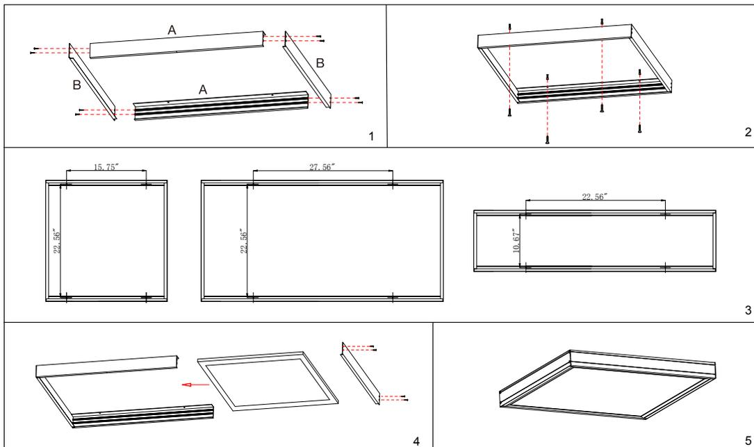
1. Remove accessories from the package carefully. Put together the four-piece surface mount kit by using the supplied ST4\*8 Cross countersunk head self tapping screws. (Fig 1)
