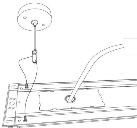
1. Screw the hanging cable to the fixture (see Fig.1)
