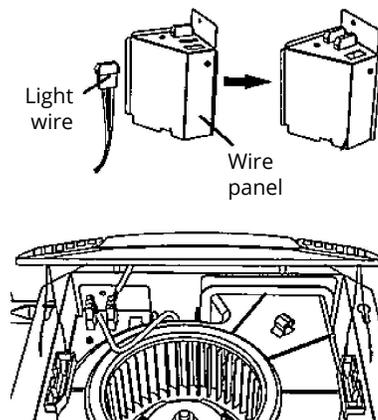
1. Remove the wire panel. Insert the light wire into wire panel. Connect electrical wiring while referring to the diagrams from the WIRING section below
