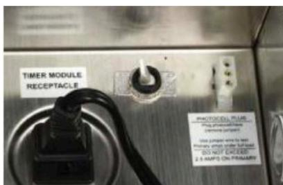
Unplug the jumper connection from the transformer
