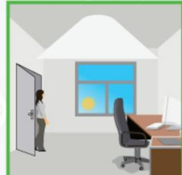
The light switches on automatically with presence when natural light is insuficient.
