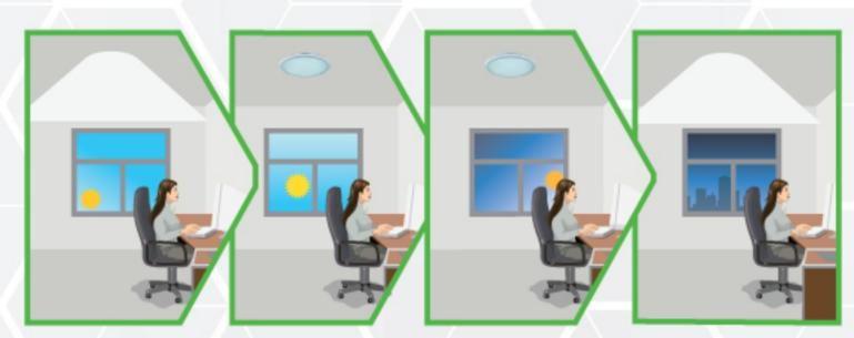
The light turns on at full or dims to maintain the lux level. The light output regulates according lathe level of natural light available.
