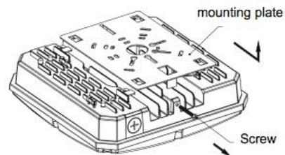
2. Use screws to lock the mounting plate onto the embedded junction box.
