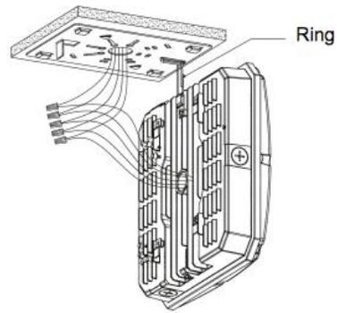
4. Align the fixture with the mounting plate.
