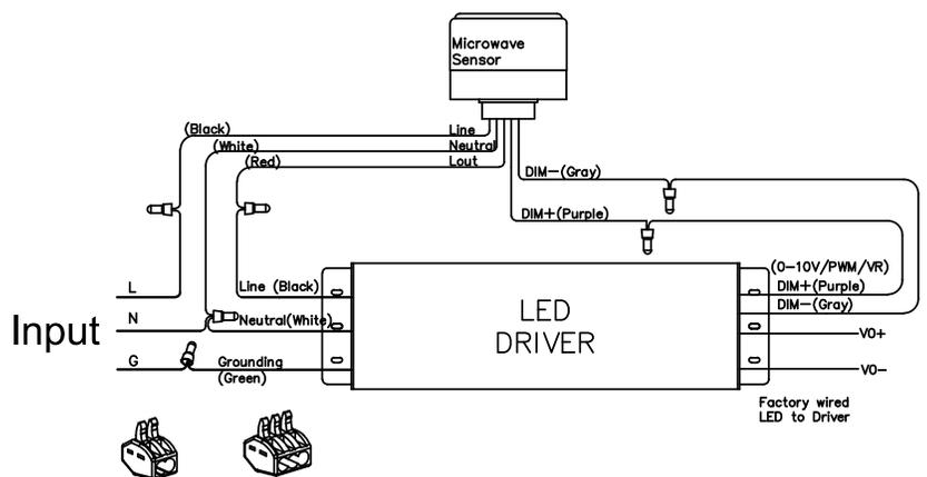
4. Connect the wires according to the wiring diagram. Wago connectors are recommended.
