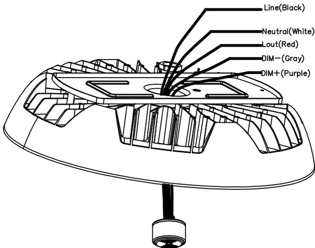
3. Insert the motion sensor through the 1/2" knock out, then screw on the lock nut.
