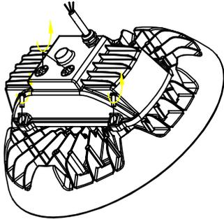
1. Detach the driver box by unscrewing the 4 screws.
