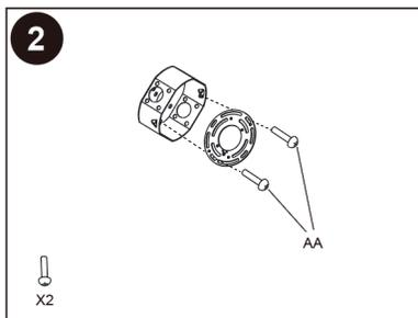
Insert long screws (AA) into aligned holes and then tighten.
