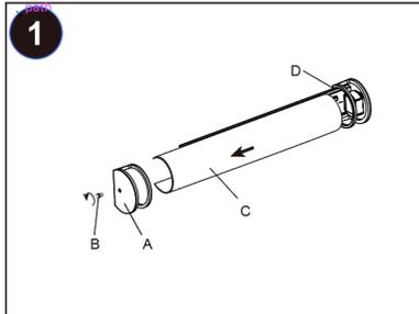
Remove the ring (A) from the fixture by loosening the mount screw (B), then remove the lens (C) from the fixture housing (D).
