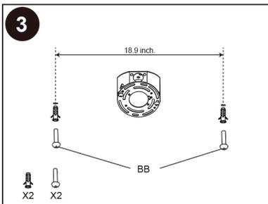
Position the fixture over the junction box and mark the location of the two keyhole slots located on the fixture housing. Be sure to mark only the narrow parts, then drill the two holes using an appropriately sized drill bit. Insert the provided anchors into the holes, then insert long screws (BB) into anchors, leaving about 1" of space between the screw heads and anchors.
