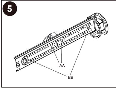
5 Locate the fixture housing (A) over the outlet box, put the long screw (AA) through the long hole slot on the fixture housing (A) and thread into the outlet box. Align keyholes on fixture pan with long screws, then move fixture housing until the long screws (BB) engage the narrow end of the keyholes. Tighten screws (AA and BB) to secure.
