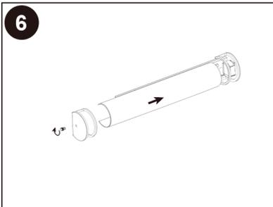
6 Secure the lens and the ring to the fixture housing by tightening the mount screw.
