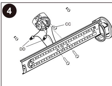
Connect the fixture wires to the supply wires: black to black, white to white, green to copper/bare/outlet by groundscrew (CC).
