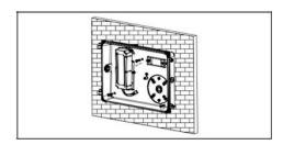
4. If wiring is performed using a recessed junction box then drill out the appropriate junction box holes. Then, line up the back plate in the desired location and mount securely. Use the supplied gaskets for a weather tight seal between back plate and junction box. Attach the driver input wires to the color matched supply wires.
