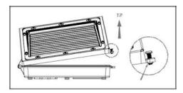
2. Wiring can be performed using a recessed junction box or a surface conduit. The fixture back plate has a template that matches two standard junction box sizes. Conduit is connected using the 1/2" NPS tapped holes ("A").
