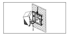
6. Fasten the front housing assembly to the back plate. Installation is now complete.
