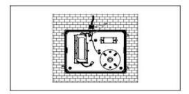
5. Line up the back plate in the desired location and mount securely. Use the supplied gaskets for a weather tight seal between back plate and junction box. Plug the male connector of the led board into the female connector of driver.
