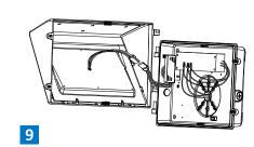
Hook the cover of the fixture onto the mounted back plate and reattach the cover connector
