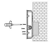
Level and secure the bottom shell on the octagon box with screws and the back plate bubble level
