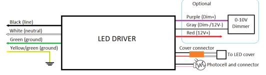
Photocell is installed in the hinge side knockout location and connected as per the wiring diagram.
