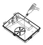
Drill holes through each of four corner mounting locations
