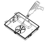
Drill holes through the back plate to match the junction box mounting screws required
