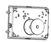
Peel and adhere large foam pad to back of mounting plate. Remove inner sections for screws
