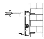
Level and secure the bottom shell with screws and the back plate bubble level
