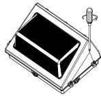
Ensuring uniform gasket coverage, close the cover and tighten Phillips screws to complete installation
