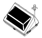
With a #2 Phillips screwdriver, loosen the cover screws
