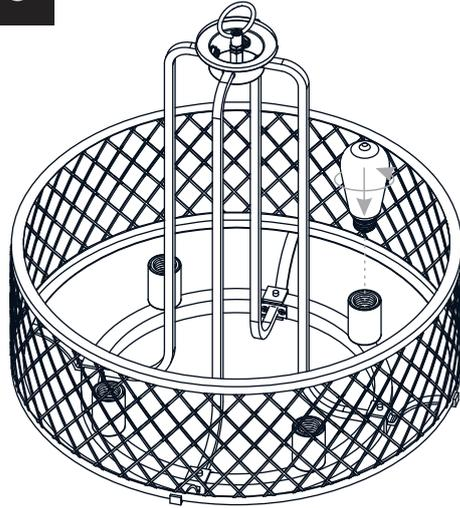
Install four correct bulbs referring to fixture markings and/or labels for maximum wattage.
