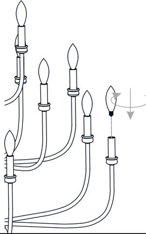
Install fifteen correct bulbs referring to fixture markings and/or labels for maximum wattage.
