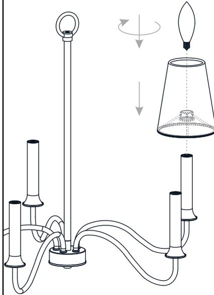
Install five correct bulbs referring to fixture markings and/or labels for maximum wattage.
