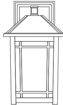
Fixture can only be mounted in the direction indicated
