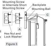
Assembly (A) by unscrewing the preassembled hex nut and lock washer and then screwing the mounting screws or alternate short mounting screws in or out of the crossbar until the correct length is achieved. Once the backplate on Fixture Body (C) is secure, remove the mounting ball and Fixture Body (C) and proceed to Step 4.
