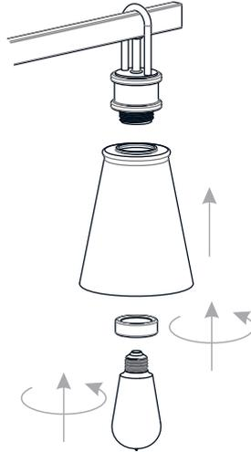
Install five correct bulbs referring to fixture markings and/or labels for maximum wattage.
