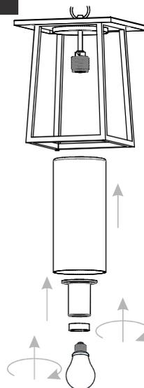
Install the correct bulb referring to fixture markings and/or labels for maximum wattage.
