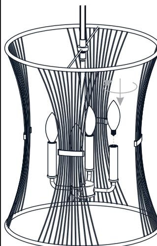
Install four correct bulbs referring to fixture markings and/or labels for maximum wattage.
