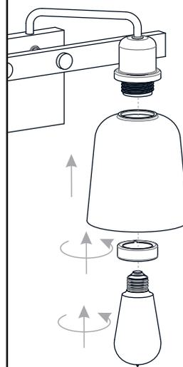
Install two correct bulbs referring to fixture markings and/or labels for maximum wattage.
