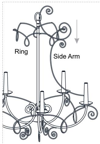
3. Screw out the set screw on the holder underside of the socket cap with Allen wrench. Insert the bottom end of the side arm into the holder. Secure by threading the set screws back in the holder. Hand tighten until snug.
