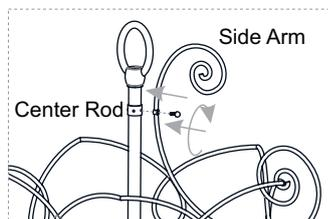
4. Attach the top end of the side arm to the center rod and secure with the lock screw. Hand tighten until snug.
