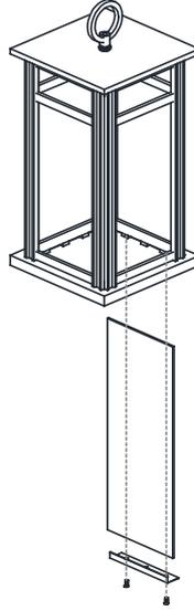
Reverse above steps to reinstall the replacement Glass Panels onto fixture.
