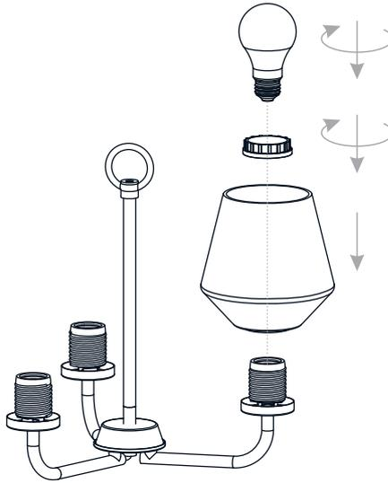
Install three correct bulbs referring to fixture markings and/or labels for maximum wattage.
