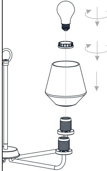
Install five correct bulbs referring to fixture markings and/or labels for maximum wattage.
