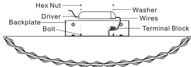
C. Connect the Live Wire from Driver to Port "L" on the Terminal Block, which is the corresponding port of the Live Wire from LED Panel. Connect the Natural Wire from Driver to Port "N" on the Terminal Block, which is the corresponding port of the Natural Wire from LED Panel.
