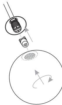
Install six correct bulbs referring to fixture markings and/or labels for maximum wattage.
