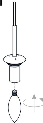
Install six correct bulbs referring to fixture markings and/or labels for maximum wattage.
