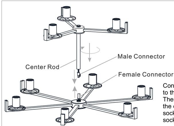
Connect the male connector to the female connector first. Then tuck all slack wires into the center rod and install top socket assembly to bottom socket assembly.
