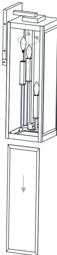
Reverse above steps to reinstall the replacement Glass panels onto fixture.
