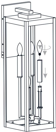
Install four correct bulbs referring to fixture markings and/or labels for maximum wattage.
