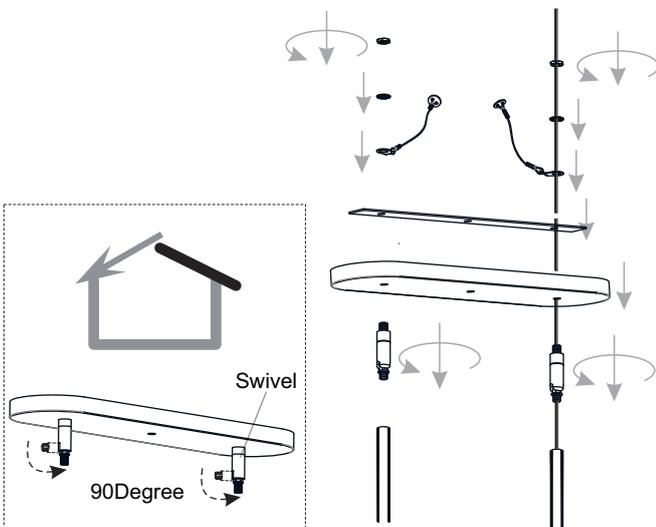
\* Make sure two swivels opening are in the same direction while assembling.
