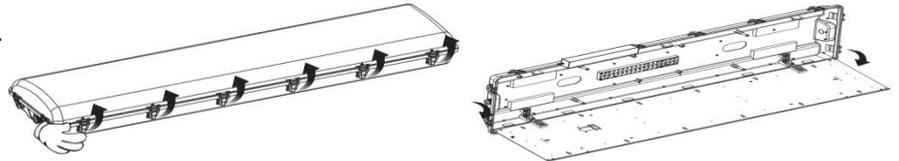
3. Attach the back housing to the stainless steel hook brackets.
