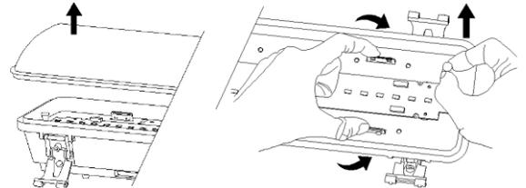
Attach the back housing to the stainless steel hook brackets.
