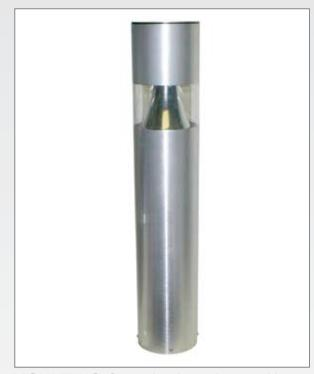
**MOUNTING** Cast aluminum base with four galvanized steel anchor bolts (1/2" x 12"). Lower body is secured to base with stainless steel screws.
