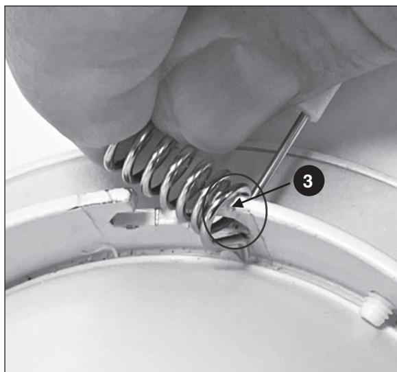
**STEP 3: The spring coil must be inserted into the fixture trim cutout support tab; by compressing the spring coil so it engages into the Left or Right cutout support tab of the fixture trim, see Figure 3.**
