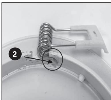
**STEP 2: Insert the 45° tail of the spring coil into the left or right cutout support tab of the trim frame, see Figure 2.**
