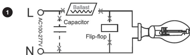
**STEP 2:** Make sure the Alternating Current Wires connect to the EX39 socket directly. Reattach or replace ground lead if one is needed. See Figure 2.
