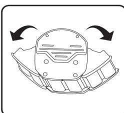
Adjust lamp so center panel is facing toward the front, then unfold side panels down.
