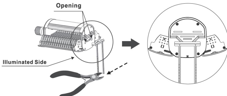
**WARNING: Both sides of the lamp must be extended in order to operate.**
