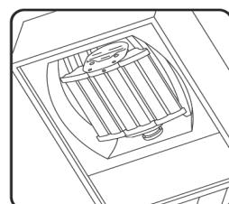
Finish the installation with the mounting bracket and replace the fixture lens.
