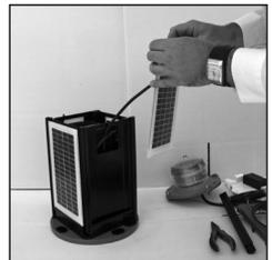
The replacement of a solar panel should only be performed by a confident technician. Sealite cannot guarantee the chassis will remain waterproof, if it not performed by Sealite staff. To test for any leaks remove the gore vent and pressurise the assembled Light to 1.5psi.
