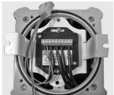
SL10 AMP Regulator shown when correctly fitted
