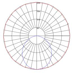
$\label{eq:maximum} \begin{array}{ll} \text{Maximum Candela} = 1671.01 & \text{Located At Horizontal Angle} = 10, \text{ Vertical Angle} = 5 \\ \#\ 1 & \cdot \text{Vertical Plane Through Horizontal Angles} & (0 \cdot 190) & (\text{Through Max. Cd.}) \\ \#\ 2 & \cdot \text{Horizontal Cone Through Vertical Angle} & (5) & (\text{Through Max. Cd.}) \\ \end{array}$
