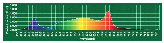
TCP's full spectrum technology provides a balanced blend of blue, green, and red light to ensure plants grow healthy and strong. The substantial red peak at 660nm results in a robust photosynthesis contribution. A blue peak shown at 440nm reduces unwanted stem elongation and leads to strong, healthy, and compact plants. Lastly, TCP's full spectrum includes a stable amount of green light, removing any need for green supplemental lighting when checking plant health.
