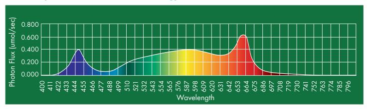
TCP's full spectrum technology provides a balanced blend of Blue, Green and Red light to ensure plants grow healthy and strong. The distinct red peak at 660nm results in a powerful photosynthesis contribution. A blue peak shown at 440nm reduces unwanted stem elongation and leads to strong, healthy, and compact plants. Lastly, TCP's full spectrum includes a generous amount of green light, removing any need for green supplemental lighting when checking plant health.
