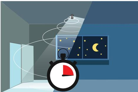
If no motion is detected and Hold Time has elapsed, lamp will set to Stand-By Dim Level.
