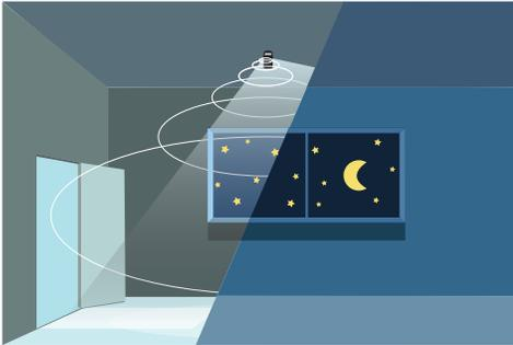
With no motion detected, lamp will set to Stand-By Dim Level.
