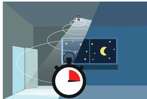
If natural light level < 300 lux, and no motion detected, lamp will set to Stand-By Dim Level.
