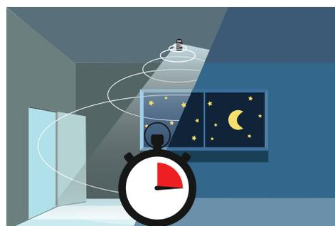
If no motion detected and Hold Time has elapsed, lamp will set to Stand-By Dim Level.
