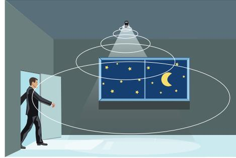
If motion is detected, lamp will turn at 100% brightness.
