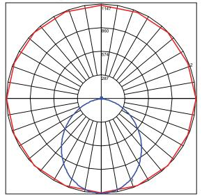
Maximum Candela = 1147.2 Located At Horizontal Angle = 0, Vertical Angle = 1 # 1 - Vertical Plane Through Horizontal Angles (0 - 180) [Through Max. Cd.] # 2 - Horizontal Cone Through Vertical Angle (1) [Through Max. Cd.)
