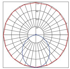
$\label{eq:maximum Candela = 1147.2 Located At Horizontal Angle = 0, Vertical Angle = 1 \\ \#\ 1 - Vertical Plane Through Horizontal Angles (0 - 180) [Through Max. Cd.] \\ \#\ 2 - Horizontal Cone Through Vertical Angle (1) [Through Max. Cd.] \\$
