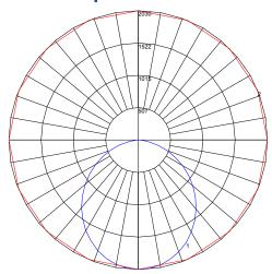
$\label{eq:maximum} \begin{array}{ll} \mbox{Maximum Candela} = 1671.01 & \mbox{Located At Horizontal Angle} = 10, \mbox{Vertical Angle} = 5 \\ \# \ 1 - \mbox{Vertical Plane Through Horizontal Angles} & (0 - 190) \mbox{ [Through Max. Cd.]} \\ \# \ 2 - \mbox{Horizontal Cone Through Vertical Angle} & \mbox{(5)} \mbox{ [Through Max. Cd.]} \\ \end{array}$
